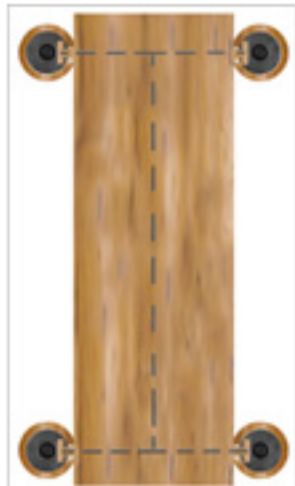
plan section; shelf and bamboo rods
