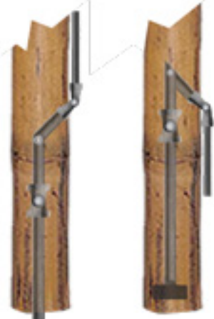
section elevation: shelves and bamboo rods; steel supports both within rod and under shelf
