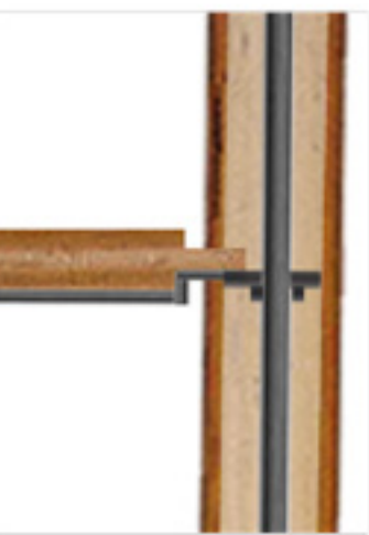
section elevation: shelves and bamboo rods; steel supports both within rod and under shelf
