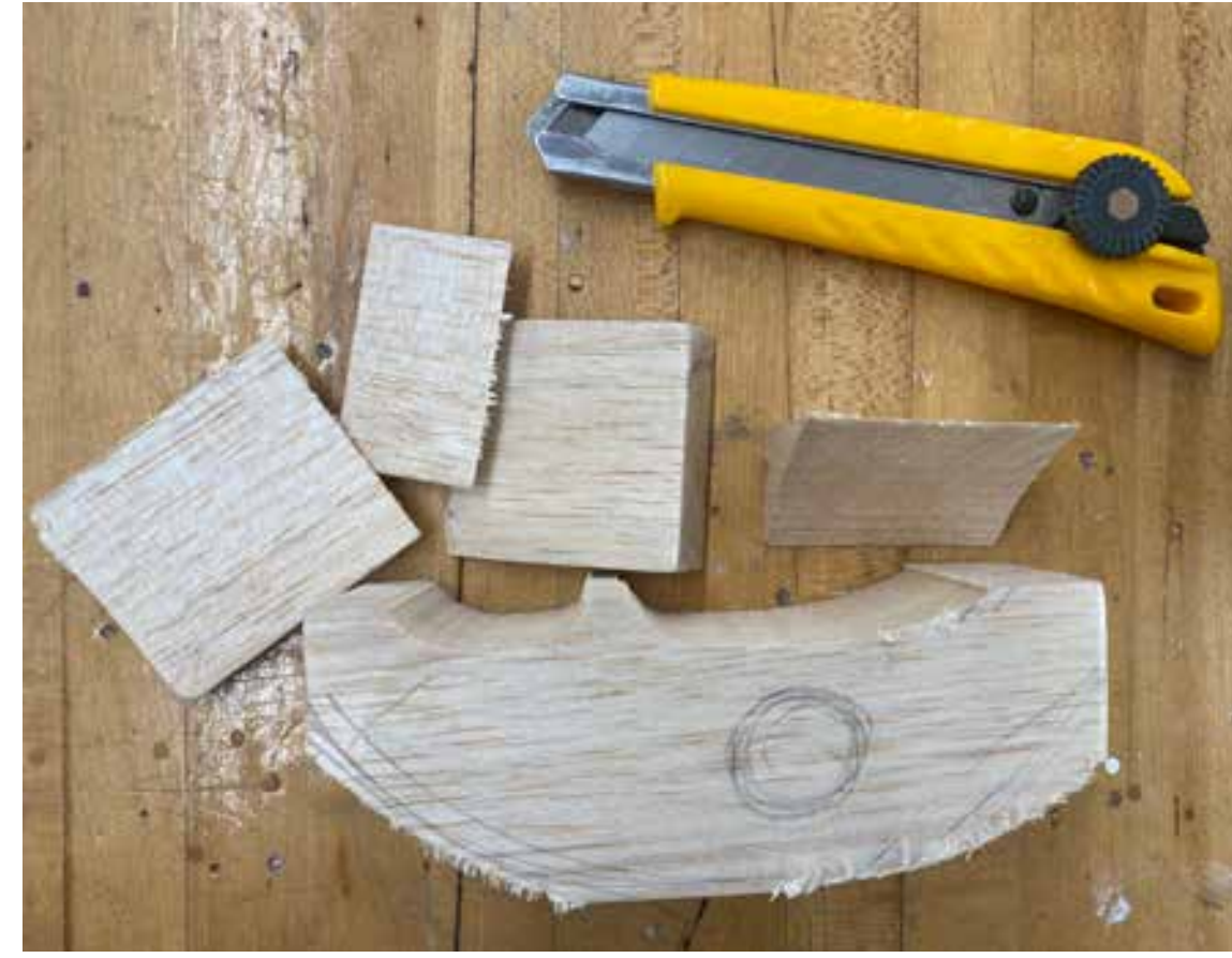
step 3 : draw and then carve with knife the right shape
